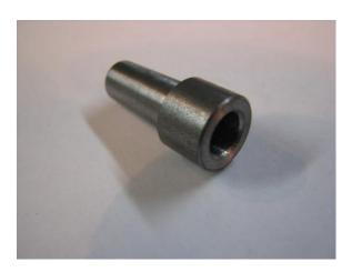
Can I still use my old UNIMAT accessories? Yes, you can. The new spindle comes with a M12-1.0 mm threaded end at the spindle head. Thus all screw-on type accessories can be used. In addition, LatheCity offers an adapter for using straight pin UNIMAT accessories such as life centers. That adapter is a Morse #0 to ~7.2 mm straight hole adapter. We do also offer Morse #0 blanks if you want to machine yourself tailstock gizmos. Look for package offers.
